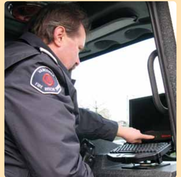
John Wilson, communications trainer for Vancouver firefighters, uses the new i/CAD mobile workstation. Laptops provide firefighters with a GPS location system, direct access to a record management system and real-time updates of events in progress.
