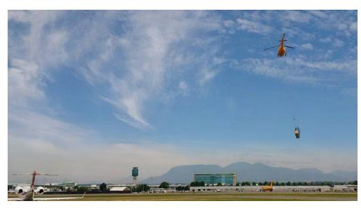
Helicopter en route to deliver a Motorola P25 radio rack from YVR to an E-Comm radio site.
